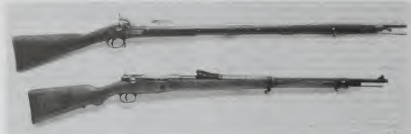
Figure 11: Two manually operated infantry rifles of the 19th century. (Top) The British Enfield Pattern 1851, a percussion-ignition, Minié-type muzzle-loader. (Bottom) The German 1898 Mauser, a bolt-action, magazine-fed repeater.
